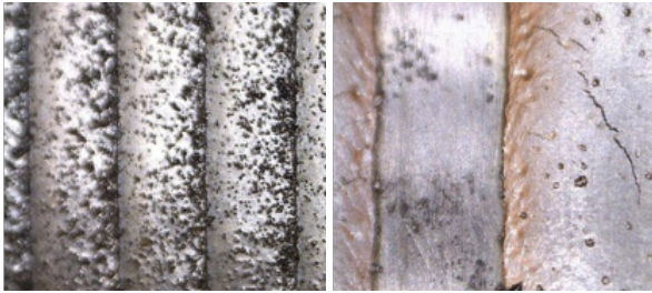
Surface of a pure cobalt-chrome cladlayer (left), crack formation in martensitic stainless steel (right).
